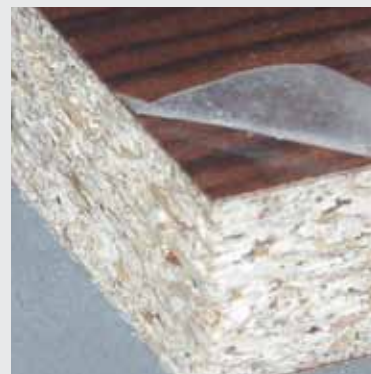
Clean edges: high gloss laminate machined with the LEUCO „PowerTec III“! The sample was even machined by using a protection foil.
