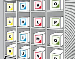
On the motor spindles signs with the corresponding colours and letters will be placed. The classification of rack, tool and motor will be extremely simplified. This system can be applied without any tooling or production know-how if necessary. New staff employed by the parquet manufacturer can easily find its feet.
