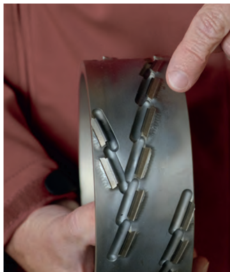
LEUCO p-System 70 shear angles enable a "pulling" cut
