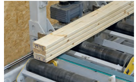
The finished planed profiles have a tolerance of 2/100 mm over lengths of up to 15 m.
