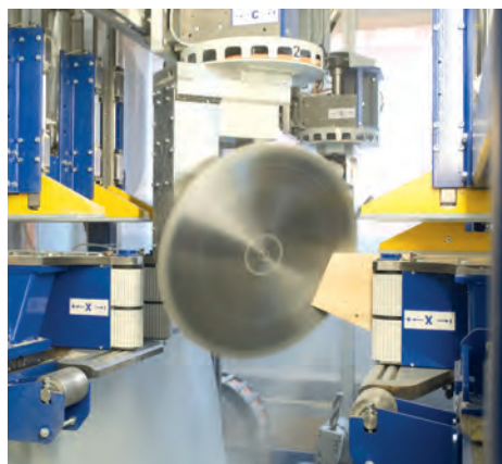
The tools can be controlled in five axes.
