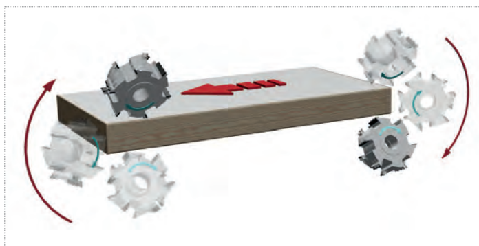
Schematic view of the machining of veneer edges - upper corner with the feed.
