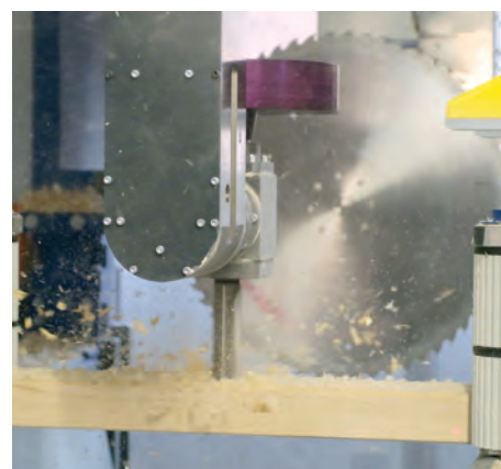
The workpiece is moved, the unit carrier is stationary.
