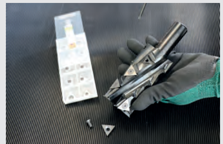
With an Allen key, all 18 knives can be removed, cleaned and replaced in 10 to 15 minutes.
