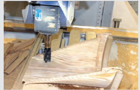
The cutter is optimally suited for freeform surfaces, as spiral and inclined cutting is possible.
