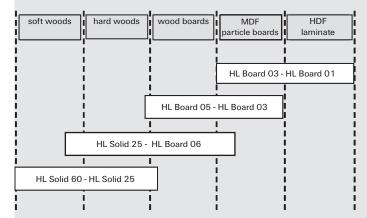
The spectrum of tungsten carbide grades ranges from HL Board 01 to HL Solid 60. HL Board grades are hard and wear-resistant. HL Solid grades are tougher and can have a smaller wedge angle.
