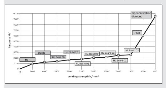
This suggests that an increase of hardness is inevitably linked with a decrease of the bending strength. With other words: "Hard cutting materials need a large wedge angle."
